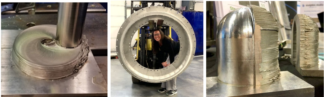
Fig. 7. Examples of an experimental (Phillips et al., 2021) and two industrial AFSD parts (Cole, J., 2020; Stevenson, K., 2018).
