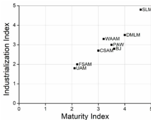
Fig. 1. Relative maturity of M-AM processes as of 2023 (Vaz et al., 2023).
