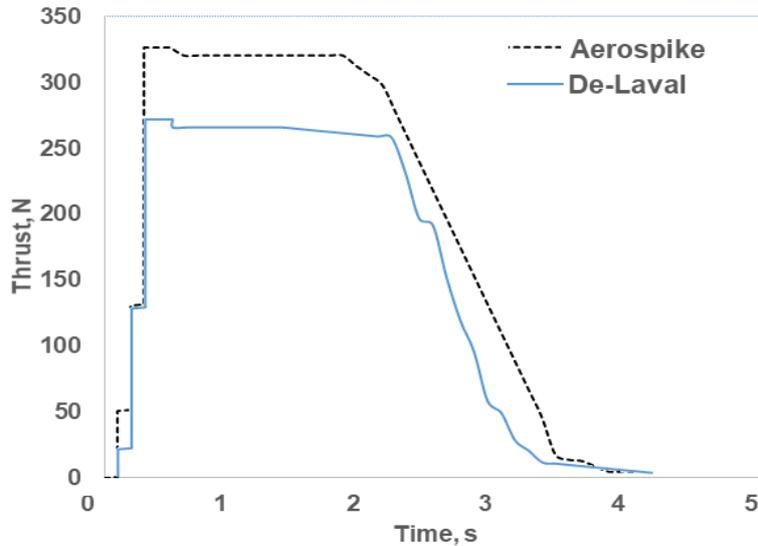
CFD analysis results revealed that the flow characteristics of aerospike nozzles were more optimized especially in terms of velocity, pressure and temperature distributions. The aerospike configuration produced approximately 18.5% higher thrust force compared to the De Laval nozzle and provided more efficient gas flow. De Laval nozzle, on the other hand, provided a leaner flow profile but showed performance loss due to its inability to adapt to changes in external atmospheric pressure.
